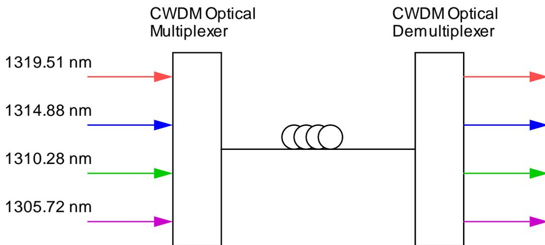
The implementation would be to vary the position of each of the wavelengths within its own pass band.
