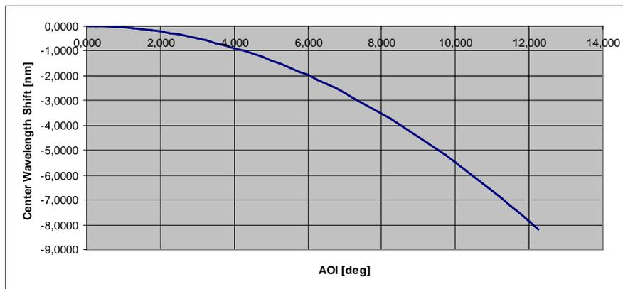
On the x-axis is the angular variation expressed in degrees. On the Y-axis is the shift in pass band. If we look at the nominal value of 10 degrees, the value of the center wavelength shift is approximately -5.5 nm. The chart below shows the region around 10 degrees where the slope of the angular variation vs. CWL shift is approximately linear.
